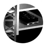
Plywood sheets, intended for assembling of the formwork on the following floors, should be arranged to be hoisted by a crane to the floor above.
